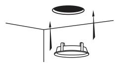
**2.** Loosen the flange clamping screws one turn (counter clockwise) to release the clamp. Next, tighten all four flange clamp screws evenly to secure the flange to the drywall. It is best to tighten each screw with the same amount of force (torque). **CAUTION:** Do not over-tighten.
